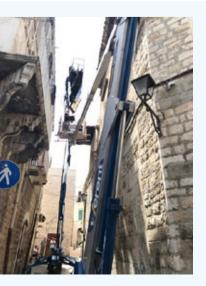
The Palfinger P160 is a high-performance truck platform. With its articulated arm it is able to reach a working height of 16 meters. The narrow and compact carriage, together with its capacity to stabilize without going out of its frame, makes it a versatile and particularly performing machine even in small spaces.
