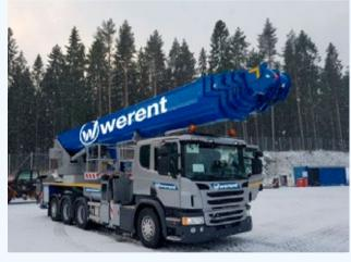
The Bronto S 70 XR is a high-performance machine. With a horizontal reach of up to 37 metres and a working height of up to 70 metres, it is a machine that specialises in lifting personnel, while maintaining the highest safety standards, also thanks to its nacelle which is capable of rotating up to 180 degrees. The S 70 XR is not characterized as exceptional transport, in fact the machine does not
